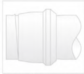
Fig. T50 — Ferrule cocked on tube
