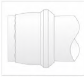
Fig. T47 — Tube not bottomed
