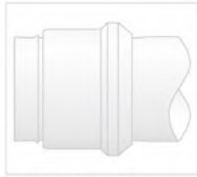
Fig. T48 — Shallow bite
