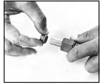
Step 2 – Slip nut and ferrule over deburred tube end. Be sure the long, straight end of the ferrule points toward tube end.
